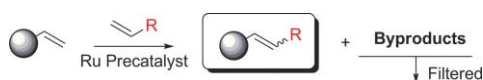
Scheme 2 Solid-supported version of olefin cross metathesis. Potentially, most of the olefin by-products generated during the reaction can be eliminated by filtration.
